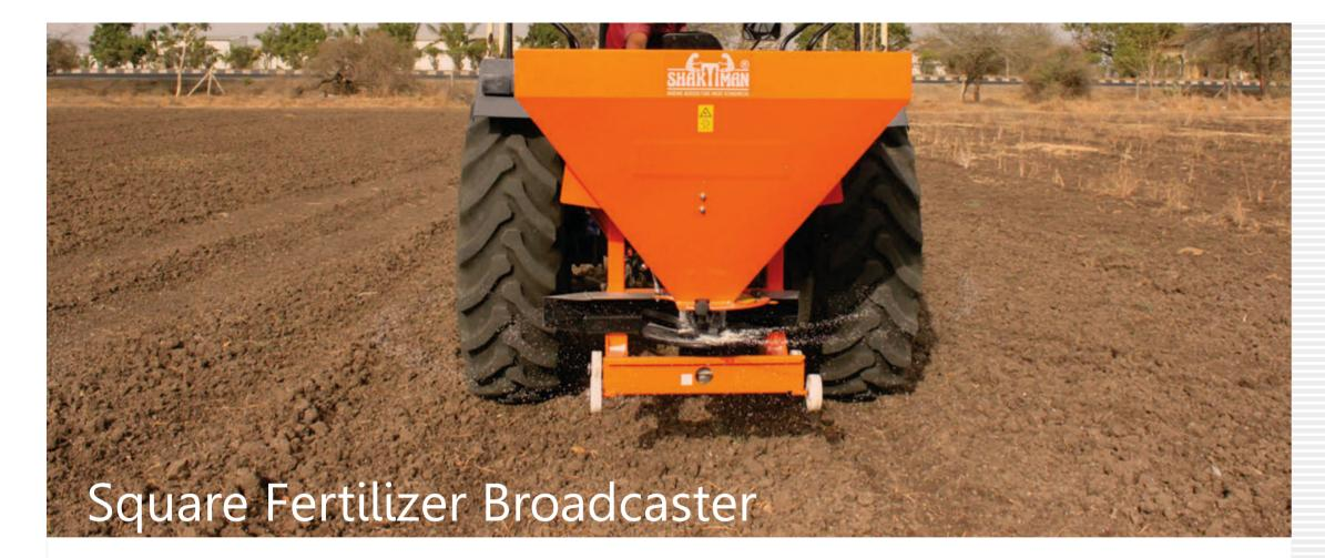
**SHAKTIMAN** Square Fertilizer broadcaster is a machine with square shape Hooper, Spreading disc system with four blades, ideal for granular or crystalline fertilizer. Its unique distributing system ensures uniform spreading of fertilizer over greater distance.
